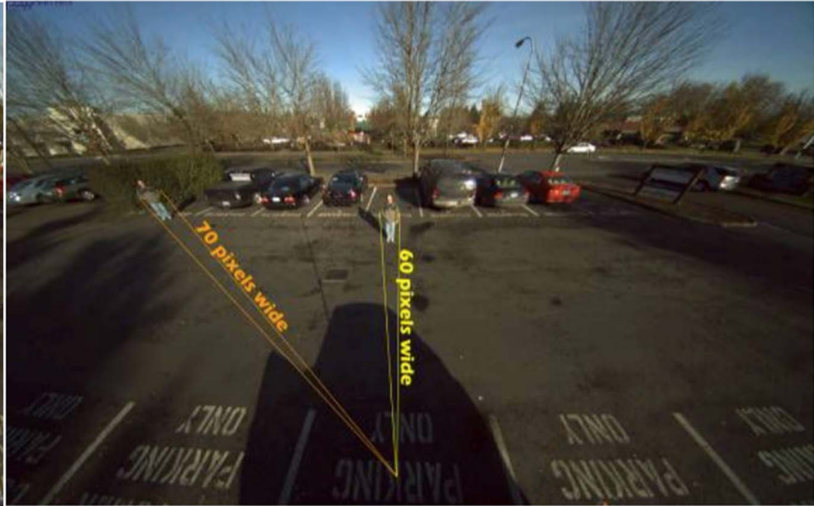
The same image taken with a rectilinear lens shows increased resolution towards the edge of the image.
