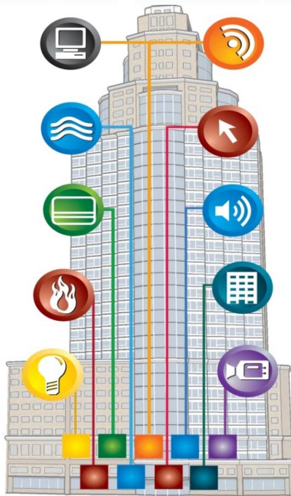
Traditional – Multiple systems, multiple proprietary cabling types
