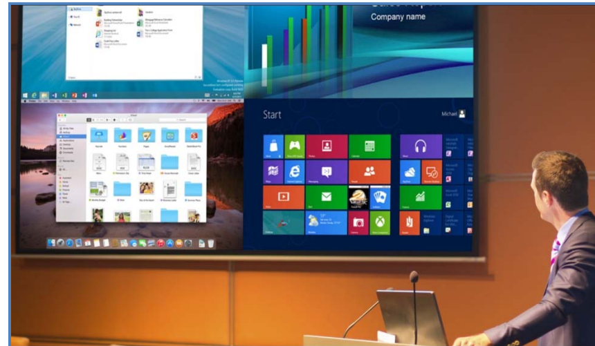
The AMX Enzo is a good example of a MirrorOp based BYOD solution. A "task specific computer" (NMX-MM-100) anchors the design.
