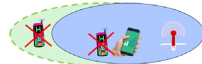
Foreign signal un-filtered, damaging uplink
