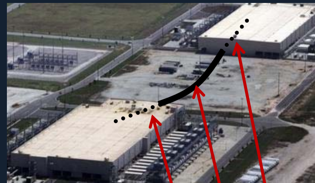
Dual Rated RR cable can avoid 1000s of splices
